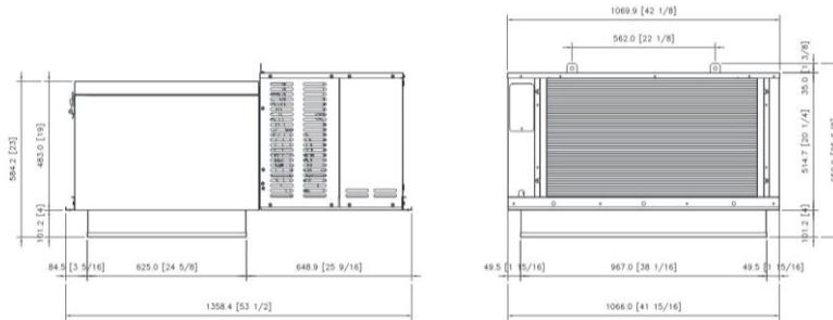
Figure C. OUTDOOR UNIT – Medium Cabinet (Opening Size : 25 inch x 25 inch) Minimum installation area ( A_{\min} ) = 6.32 m 2 ( 67.98 ft 2 )
