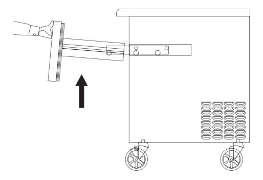
Fully extend the drawer out toward you as pictured. After full extension, lift the drawer up and pull towards you. This will disengage the rollers from the roller guide.
