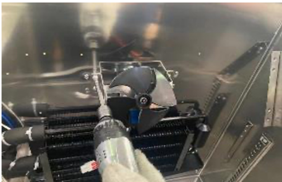
E. Remove the evaporator coil
