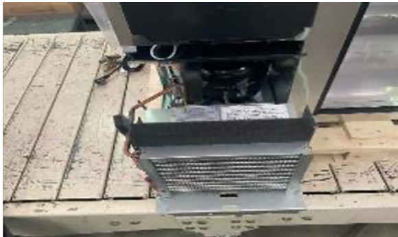
E. Disassemble the condensing unit
